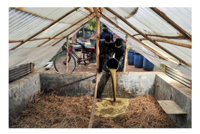
Collectors unload the waste at the composting site. Here, the waste is poured on to a drying bed containing rice straw. Transparent plastic roof panels help to raise the ambient temperature below and accelerate the drying process, which typically lasts 15 days
